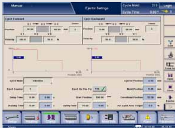
Dual ejector for separate handling of material or products.
