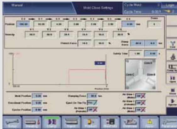
Mold protection function with 2 steps in standard.
