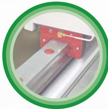
Linear guide of the rear platen of injection unit, lower friction but faster response
