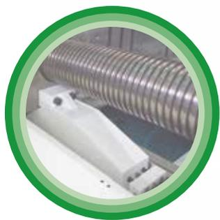
High-rigidity movable platen support device and guide mechanism on the bottom and side of machine bed ensures the precision of movable platen during loading of heavy molds
