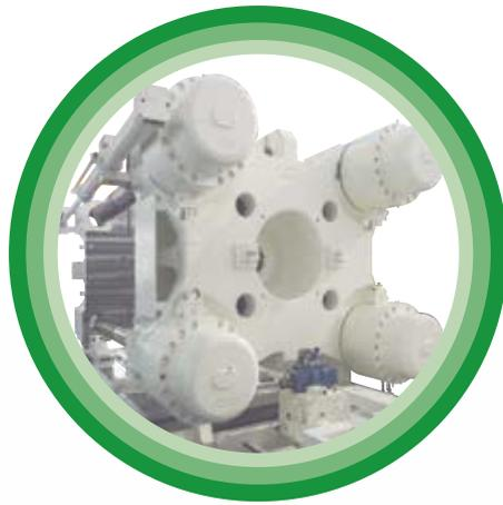
Parallel lock nut operation ensures fast and accurate response
